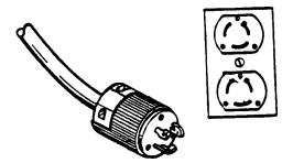
This machine must be connected to an electrically ground circuit in order to protect the operator from electric shock. This machine has an approved power cord with three conductors as well as a plug with three terminals. Connect the plug into a three holed receptacle. For maximum protection against electric shock, use a circuit that is protected by a ground fault circuit interrupter.
